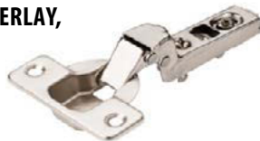
11. 110 DEGREE CLIP ON CAM, ADJUSTABLE CONCEALED EUROPEAN HINGE, INSET OVERLAY, 15MM CRANK SOFT CLOSE WITHOUT DOWELS
